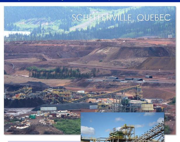
The LIM mine is an open pit with in-plant crushing, scrubbing, coarse and fine screening to fines recovery.
