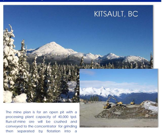
molybdenum concentrate. The concentrate will be filtered and bagged for truck transport to port facilities for delivery for offshore roasting. The project was placed on hiatus in 2015.
