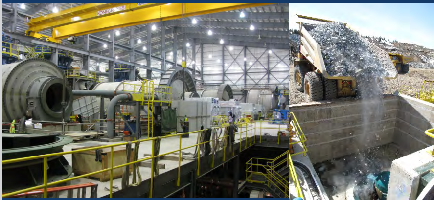
SAG, Ball (2) and Regrind Mills
